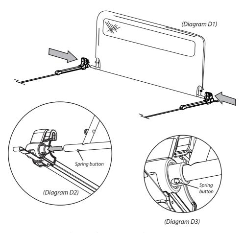
**Step 8:** Insert one side of the wall frame into one of the corner hinges. Press in the metal spring button to fully insert the tube into the hole in the plastic sleeve. (Diagram D2)
